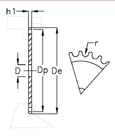
C = 4 D = 16 De = 98.1 Dp = 82.96 For chain size = 1 1/4 x 3/4 For chain type = 20 B-1 h1 = 18.5 Sumber of teeth = 8
